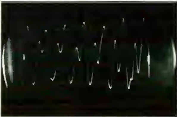
FIGURE 18—Cathode Ray Oscillograph trace of note produced by sand lying under a layer of water.
