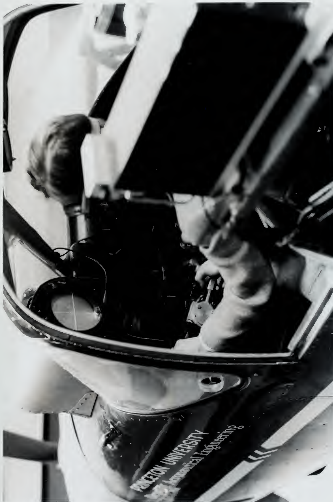
Fig. 2. Cockpit of flight simulator showing radar scope face and test pilot at the controls.
