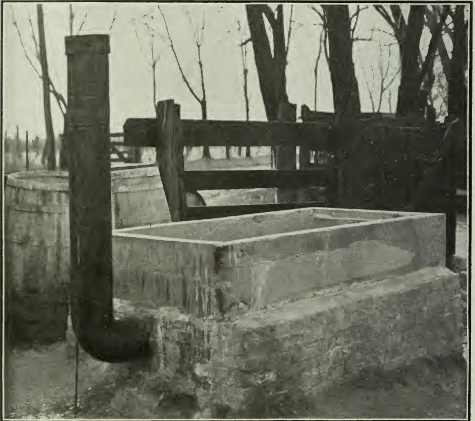
Serviceable Cooking Plant for Lime Sulphur on Farm of Robt. Thompson, St. Catharines.
