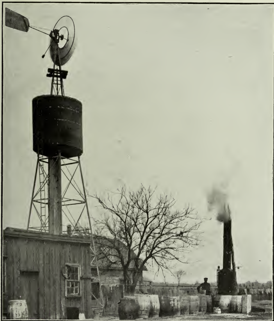
Steam Cooking Plant for Lime Sulphur on Farm of W. H. Bunting, St. Catharines.
