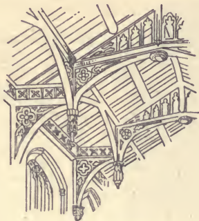
Hammer Beam Roof
