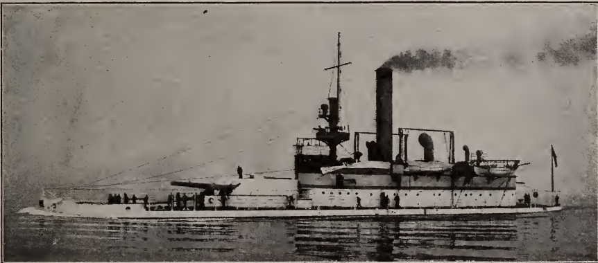
United States coast defense monitor Florida. She represents a type of vessel that marked the early improvements on Eriesson's Monitor, which was the forerunner of the modern revolving turreted battleship. Displacement, 3,235 tons; speed, 11.5 knots; guns, two 12-inch, four 4-inch rapid-fire, three 6-pounders, four 1-pounder automatic, four 1-pounder rapid-fire, two .30 caliber automatic. Although she was authorized by Congress as late as 1898, yet in 1908 she was considered so out of date and valueless as to be used as a target by the naval men.
