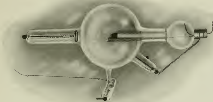
FIG. 43.—Water-cooled tube for overhead or under the couch work, showing mica and carbon regulator. (C. Andrews.)
