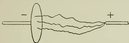
FIG. 55.—Connections of the X-ray tube to the coil, showing the route travelled by the spark when the point is the positive pole and the negative the plate.
