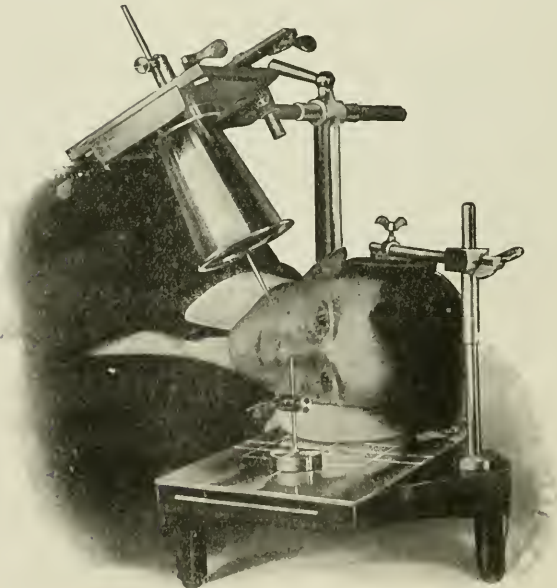
FIG. 150.—Sweet's eye localiser. Position of tube for second exposure. (A. E. Dean.)
