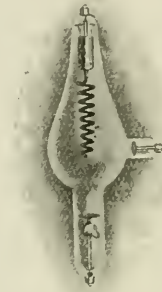
FIG. 66.—Single valve tube. (C. Andrews.)
