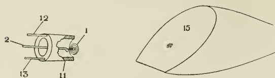
FIG. 50.—Diagram of cathode and anti-cathode of Coolidge tube.
