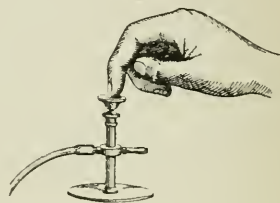
FIG. 61.—Showing method of controlling osmosis regulator from a distance.
