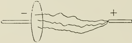
FIG. 8.—Connections of the X-Ray tube to the coil, showing the route travelled by the sparks when the point is the positive pole and the negative the plate.
