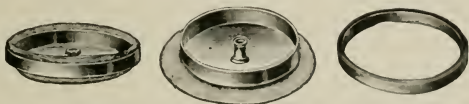
FIG. 191.—DISC ELECTRODE, WITH CELLULOID RING. The illustration on the right shows the ring only, the illustration in the centre shows the electrode with a new cover ready to be slipped over it, and the illustration on the left shows the complete electrode, with cover held in position by the ring.
