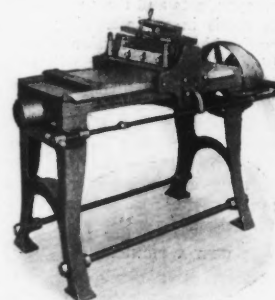
POWER SCREW DRIVEN SHAVING MACHINE Especially adapted for use in newspaper offices. The most powerful shaver made.
