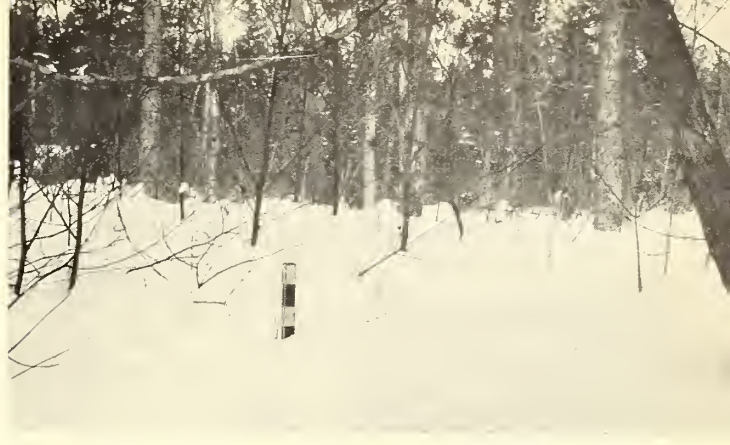
F-503690 FIGURE 10. — Snow pole in a shelterwood stand at Dukes showing 50 inches of snowpack (the 5-foot pole is marked at 3-inch intervals). A series of 60 poles observed for 4 winters showed that the average maximum snow depth increased 6 to 8 inches when the overstory was partially cut and 13 to 16 inches when it was completely removed in strips or blocks.
