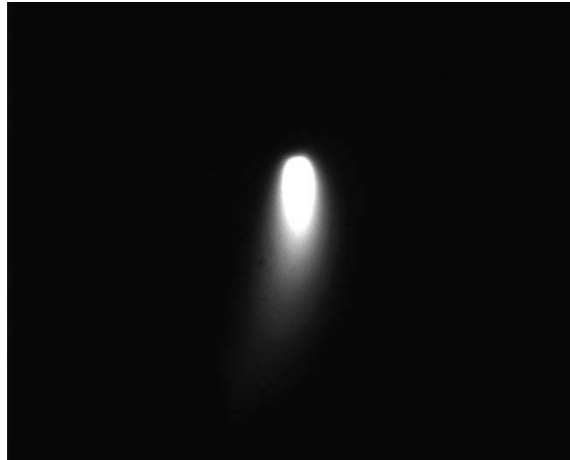
Figure 15. Spot Mode image with application of 15V DC in a specific point of a p-type AlGaAs/GaAs/AlGaAs heterostructure (216 \mu\text{m} X 190 \mu\text{m} ).
