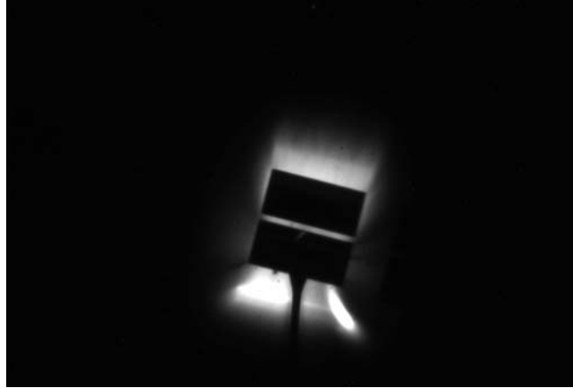
Figure 13. Picture Mode image with application of 15V AC in a p-type AlGaAs/GaAs/AlGaAs heterostructure (874 \mu\text{m} X 589 \mu\text{m} ).
