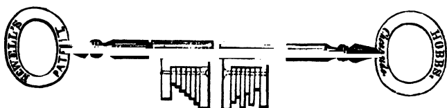
fig. 43. Key of the Parautoptic lock.
