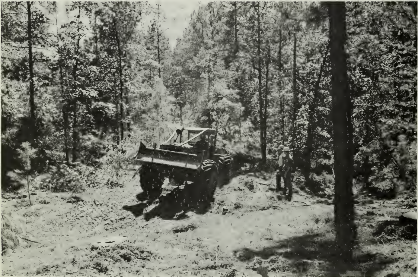
Rubber-tired logging equipment creates less disturbance of forest floor.
