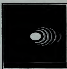
Object-glass not properly adjusted.
