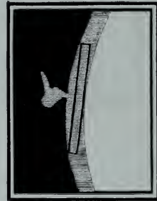
SLIT PLACED TANGENTIALLY TO VIEW A PROMINENCE.
