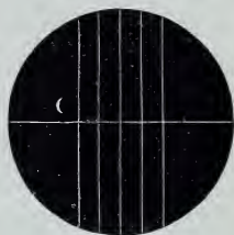
ARRANGEMENT OF WIRES IN A TRANSIT INSTRUMENT.
