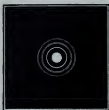
Object-glass properly adjusted.
