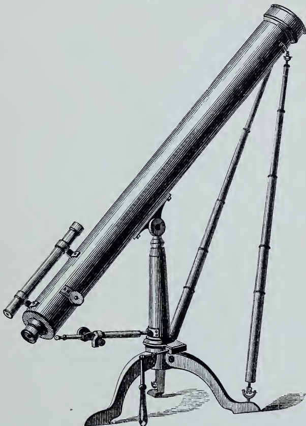
TELESCOPE MOUNTED ON A PILLAR-AND-CLAW STAND, WITH FINDER, VERTICAL AND HORIZONTAL RACK MOTIONS, (THE LATTER WORKED BY A HOOKE'S JOINT), AND STEADYING RODS.
