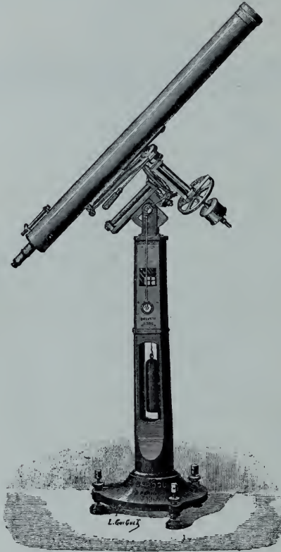
EQUATORIAL CONSTRUCTED TO ALLOW OF CONSIDERABLE VARIATION IN LATITUDE. (By Bardou. )
