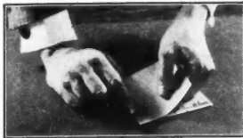
Foldability. The new Super-Safety Paper has extraordinary ability to resist sharp folding without weakening. Endurance of this sort is five times, or more, greater than that of the usual check paper. Here is a check paper that will remain crisp and fresh through the hardest service.
