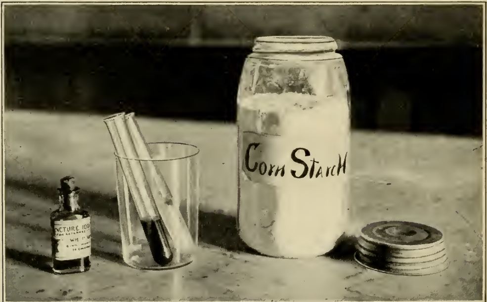
IODINE TEST FOR STARCH.
