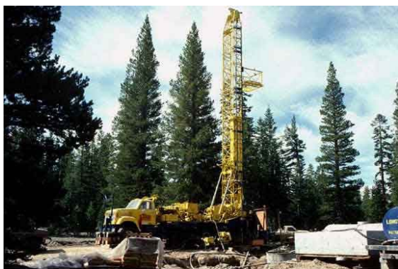
Truck Mounted Rotary Rigs are commonly used to drill temperature gradient wells.
