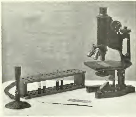
Fig. 1. Apparatus: Microscope, "hanging-drop" slides and cover-slips, wire loop and burner (or alcohol lamp), and tubes for serum and corpuscle-suspension.
