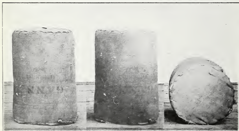
FIG. 2.—ROUND BALE, SIDE AND END VIEWS. DENSITY, 28 POUNDS PER CUBIC FOOT. APPROXIMATE DIMENSIONS, 35 BY 20 INCHES (DIAMETER).
