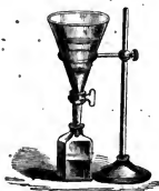
Tap funnel for separating ottos from water and spirits from oil.
