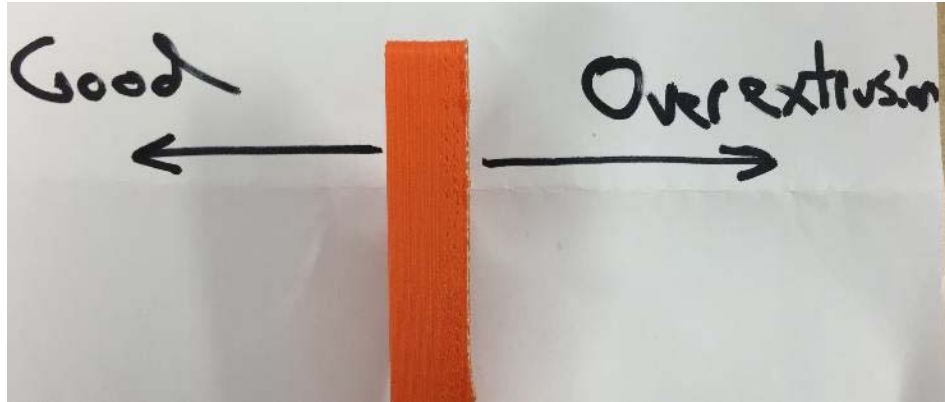
Figure 38. Correct and over-extruded extrusion rates.
