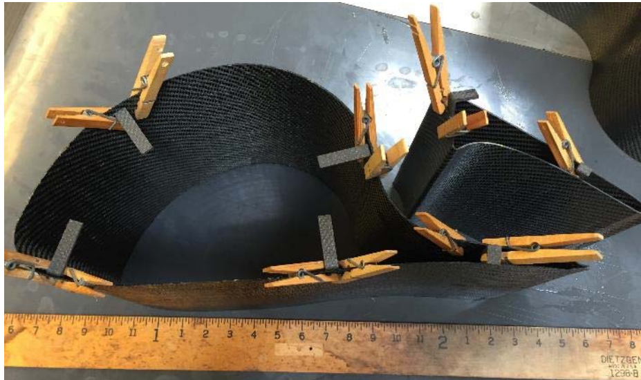
Figure 47. Wing with brackets at final spacing.
