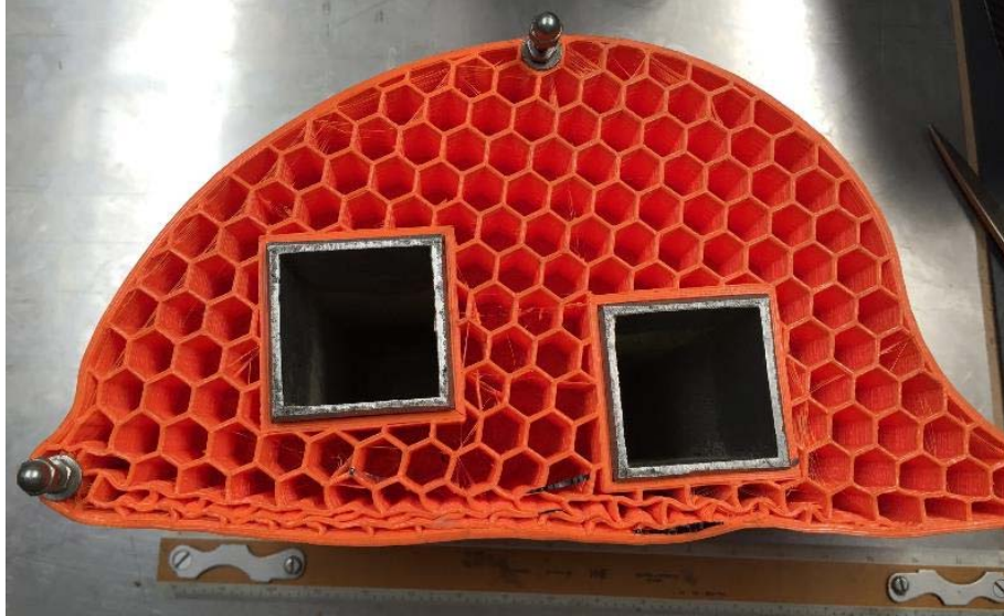
Figure 44. Local mold collapse due to radiant overheating.
