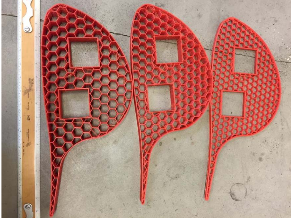
Figure 37. 10%, 15%, and 20% octagonal infill.
