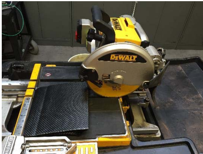
Figure 45. DeWalt tile saw used for trimming aft wing airfoils.
