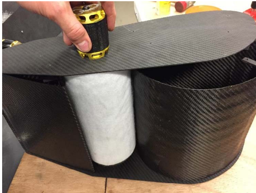
Figure 50. Felt used to properly align and space CFFs.
