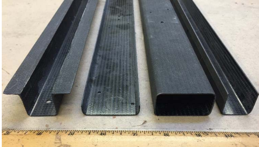
Figure 52. Potential frame member cross-sections.
