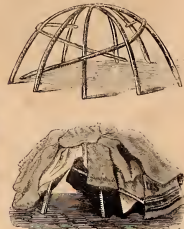
7. METHOD OF ERECTING DANDY COT.
