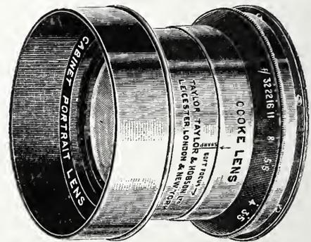
plate perfectly. A lens of this large aperture and focal length necessarily of considerable size, the glass being nearly 3½ in. diameter, and the outside diameter of the flange measuring 5½ in. The lens is supplied with iris diaphragm, whilst the front portion is capable of being separated from the back elements, so as to give a certain amount of diffusion, the makers providing an automatic stop when reverting to the sharpest possible definition. The price of this new "Cooke" is £18.
