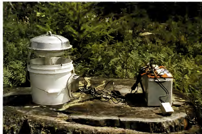
Figure 11 A light trap setup includes a containment bucket (a killing agent optional for unattended sampling), funnel, plastic veins holding the UV lightbulb, top fastened down with bungee cords, and electrical wires equipped with a photoswitch attached to a 12-volt battery. This setup can be used to sample night-flying moths for up to four consecutive nights.
