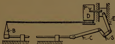
FIG. 38.—Smallwood's Drum Motion Tester.
