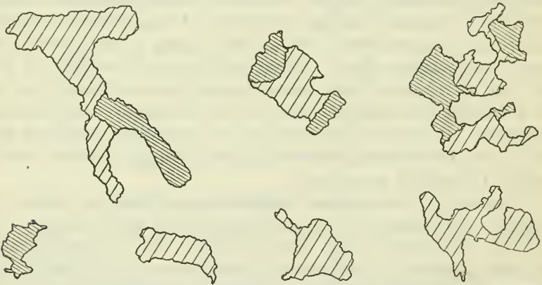
FIG. 2.—OUTLINES OF SECTIONS OF GRAINS OF IRON AND OF PYRRHOTITE FROM THE TROUP METEORITE, AS SEEN ON A POLISHED SURFACE OF THE STONE. THE CLOSELY SHADED AREAS REPRESENT PYRRHOTITE, WHILE THE LIGHT SHADED AREAS REPRESENT METALLIC IRON. MAGNIFIED ABOUT 25 TIMES.
