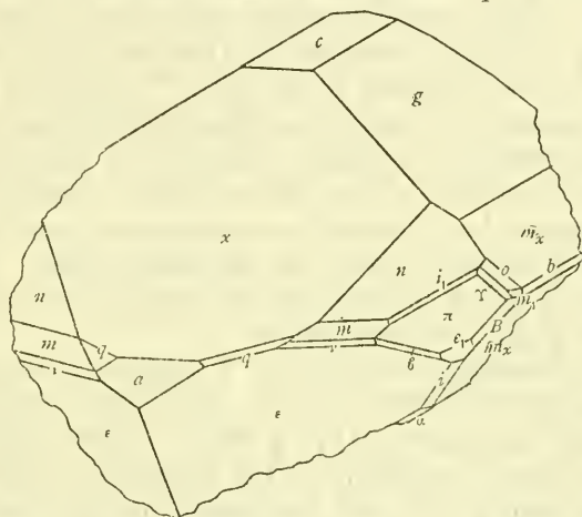
FIG. 24.—CLINOGRAPHIC PROJECTION OF CRYSTAL 33 SHOWING NEW FORMS i_1 ( \bar{4}61 ), \epsilon_1 ( \bar{3}53 ), m_1 ( \bar{1}2.25.1 ) \tau ( 351 ) AND \sigma ( 343 ).
