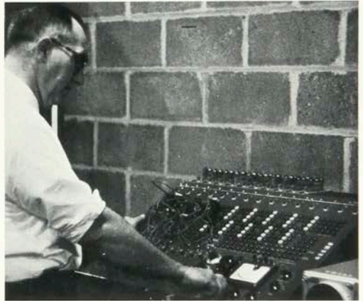
Acquisition of a Heathkit analog computer has enabled the student to make practical application of data-processing theory and circuit analysis. An intensive computer course is offered as a fifth-year elective.
