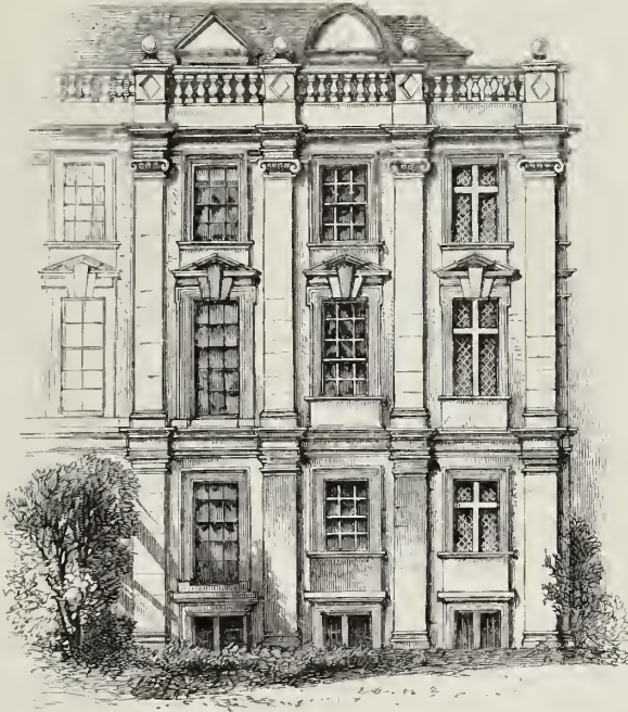
Fig. 9. River front, shewing the original design (1671), and the changes made in 1715 and 1815, reduced from a lecture diagram by Professor Willis.
