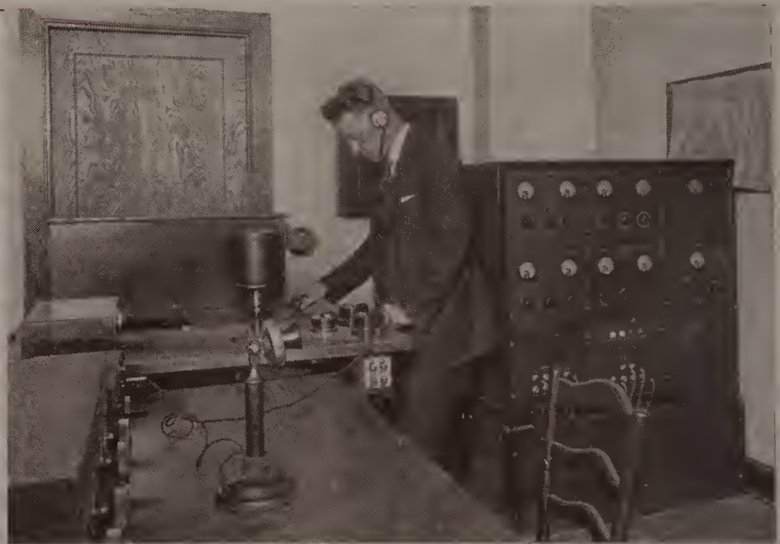
CONTROL ROOM OF DUAL STATION "WJZ-WJY" The Operator Stands before an Oscillograph—a Device for Checking the Characteristics of the Program being Transmitted.
