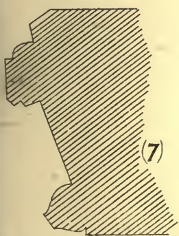
Jamb of Old Window.
