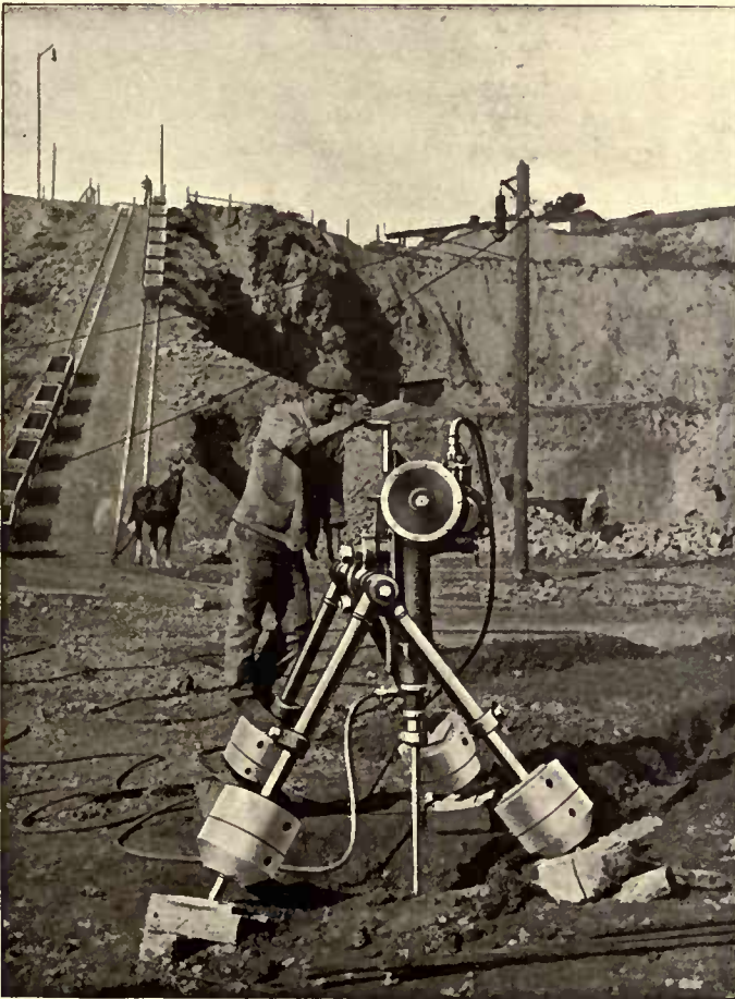
Fig. 152 Vertical Percussion Drill. With water flushing arrangement.
