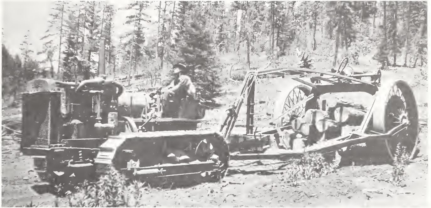
Figure 20. Ceterpillar tractor and hydraulic arch hauling logs for George E. Breece Lumber Co. or Mescalero Apache Reservation. July 1928. By J. D. Jones. USDA Forest Service photo 230661.
