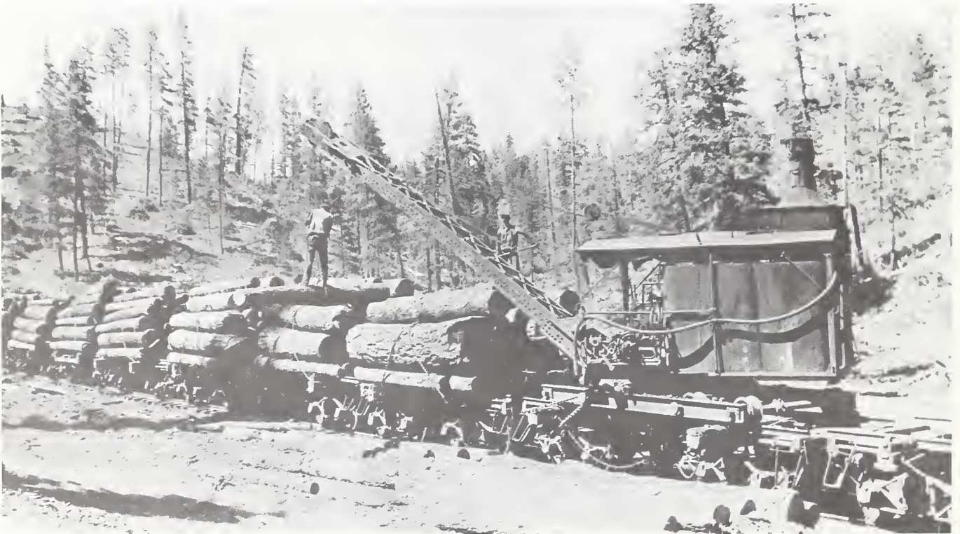
Figure 32. George E. Breece Lumber Co. loader working at landing on Mescalero Apache Reservation. The loader moves from car to car on rails permanently mounted on each car. June 30, 1928. By E. S. Shipp. USDA Forest Service photo 233085.
