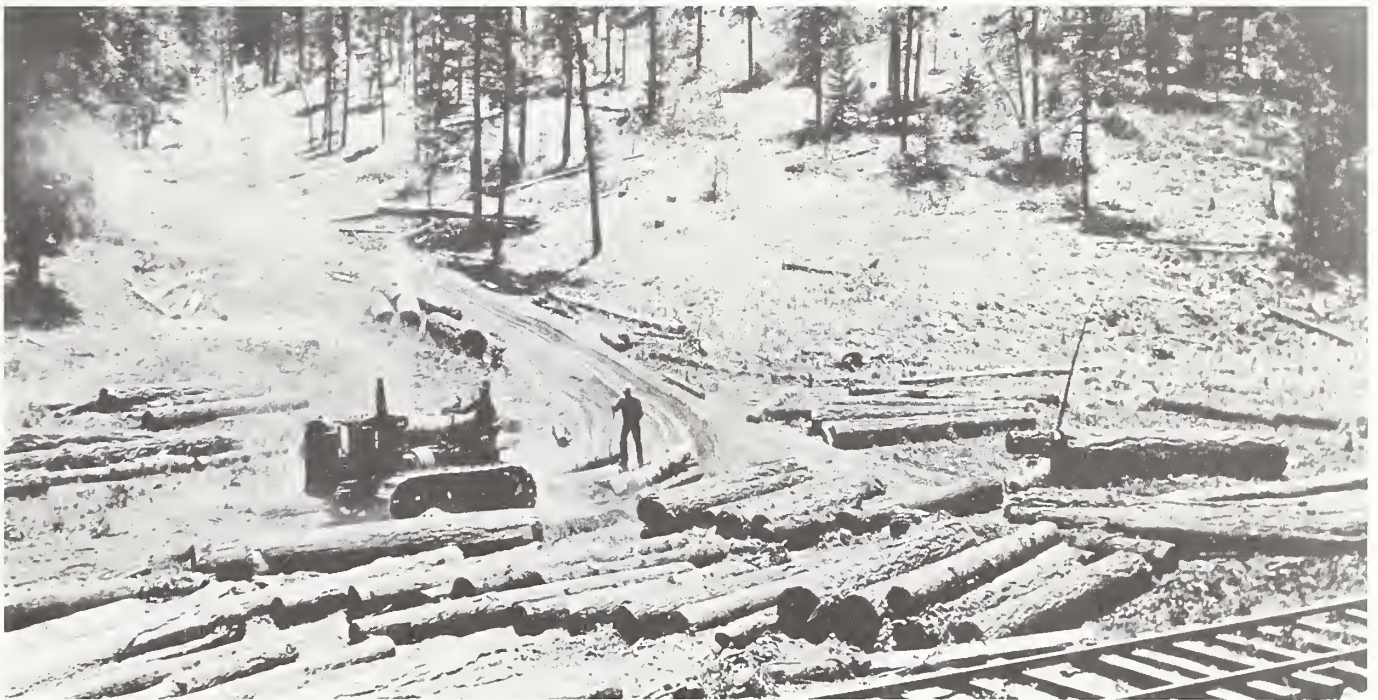
Figure 21. Skidding logs to railroad landing with Ceterpillar tractor. June 1928. Probably by E. S. Shipp. USDA Forest Service photo 233022.
