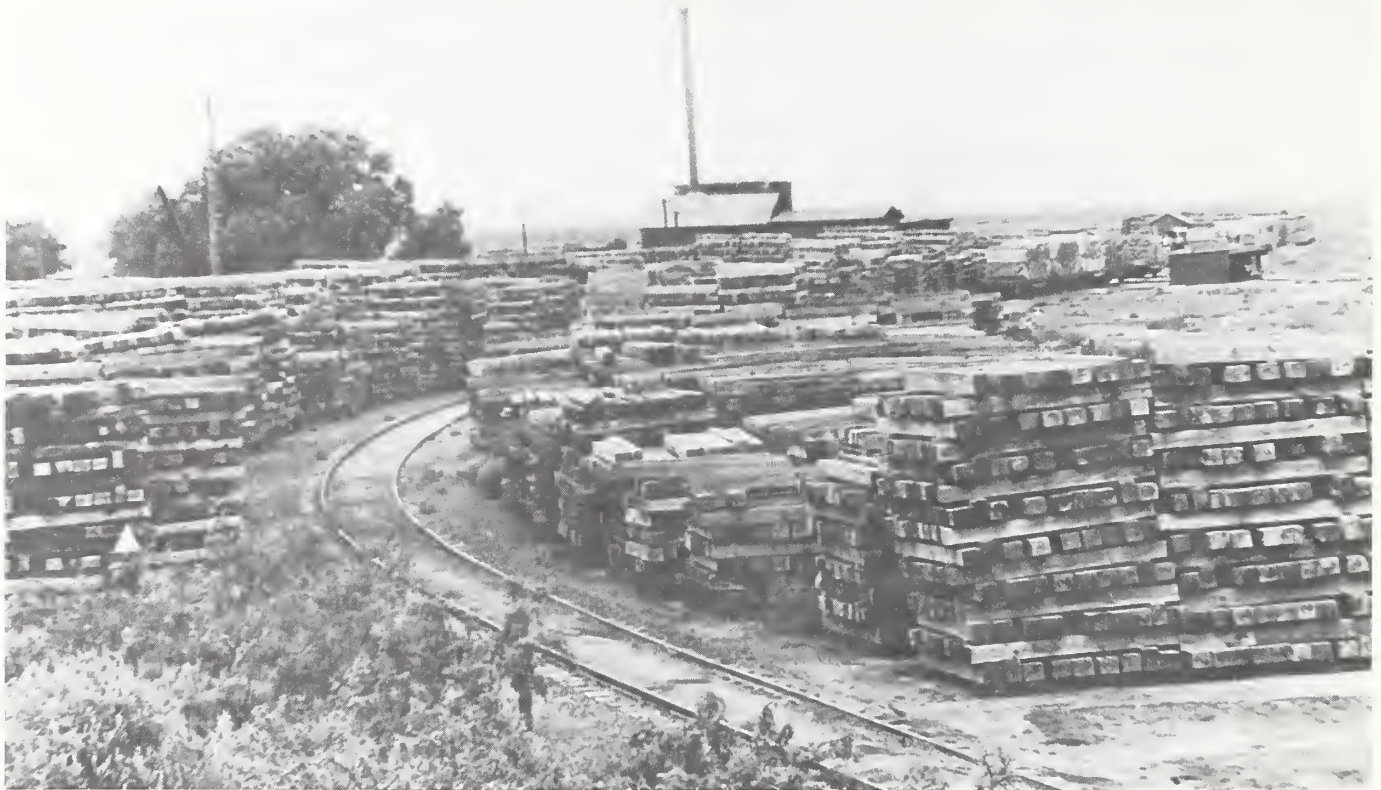
Figure 25. Southwest Lumber Co. yards at Alamogordo, with railroad ties stacked awaiting creosoting at Southern Pacific Co. treating plant nearby. July 2, 1928. By E. S. Shipp. USDA Forest Service photo 233474.
