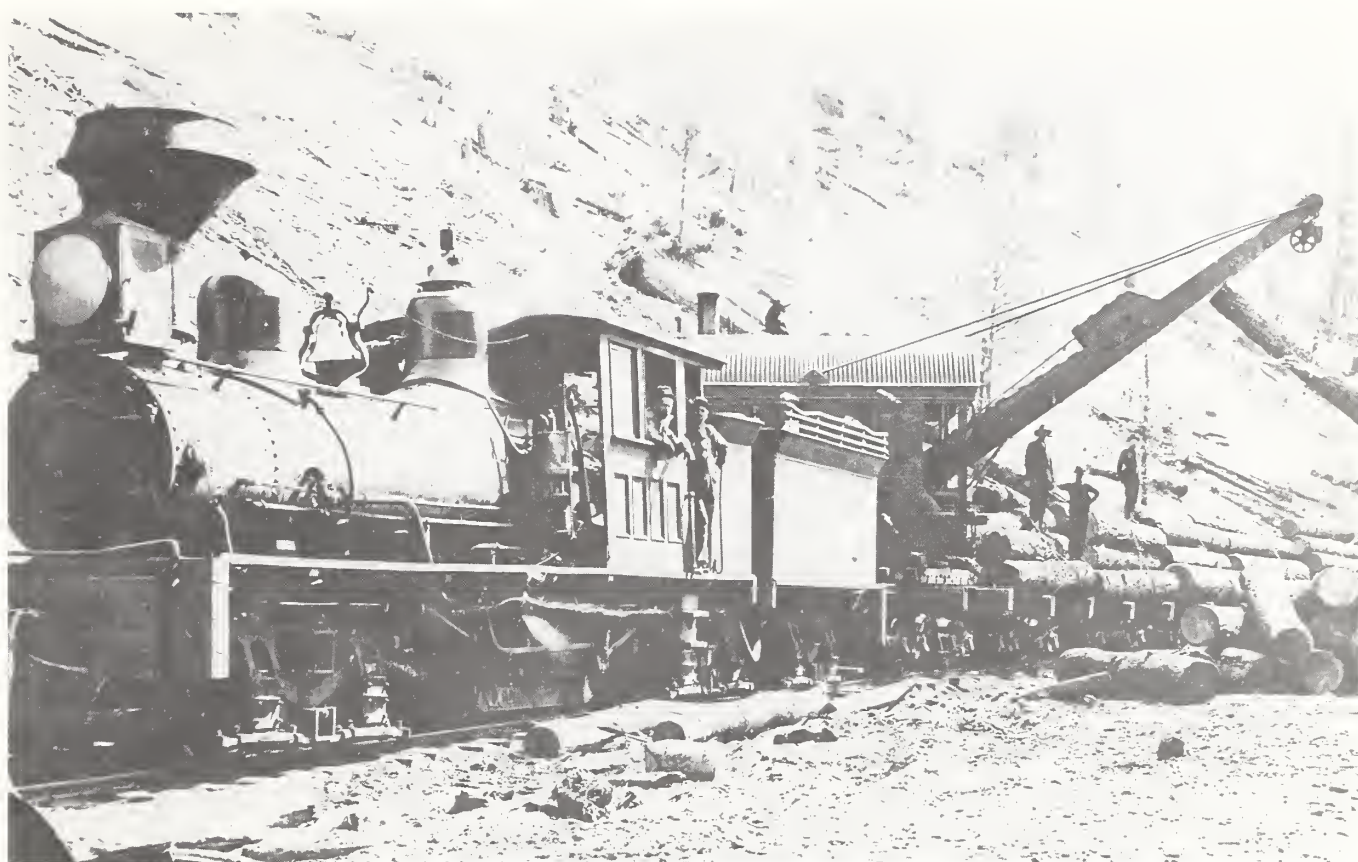
Figure 11. Alamogordo Lumber Company Shay geared locomotive and train loading logs. n.d. By Green Edward Miller. Museum of New Mexico collection.
