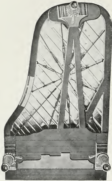
Bottom of Grand Piano showing Richard W. Gertz's Tension Resonator
