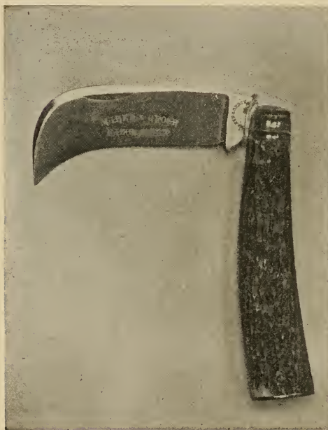
FIG. 64.—A good type of pruning knife. Long hooked blade and large enough for heavy work.
