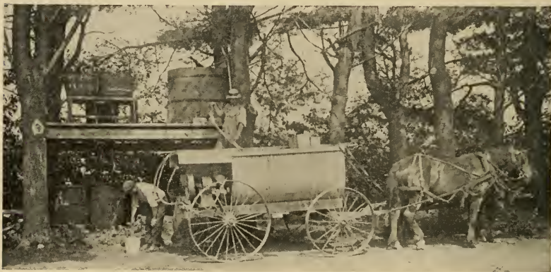
FIG. 82.—A gasoline power outfit. The most efficient power sprayer. The cut also shows an excellent arrangement for filling the tank and mixing the materials.
