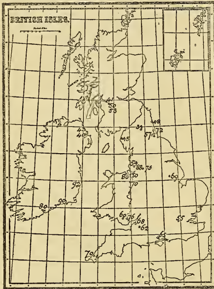
FIG. 1.—Map of the British Isles, showing the distribution of rates of increase of temperature with descent. The rates are taken from the 'British Association Report,' except in the case of those in the south of Ireland.
