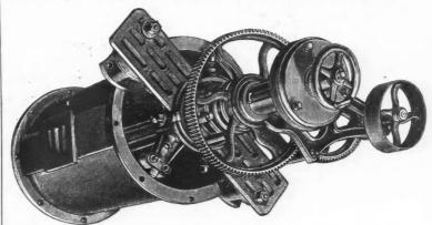
piece that is bored serves as the bed or support of the bar, making it entirely a portable tool, doing the truest of work, because no springing strains are brought on it.
