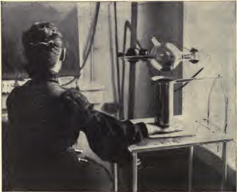
FIG. 267.—Skiagraphing hand by the aid of Beck's diaphragm.
