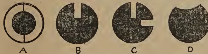
FIG. 10.—Diagram of stops for oblique illumination.
