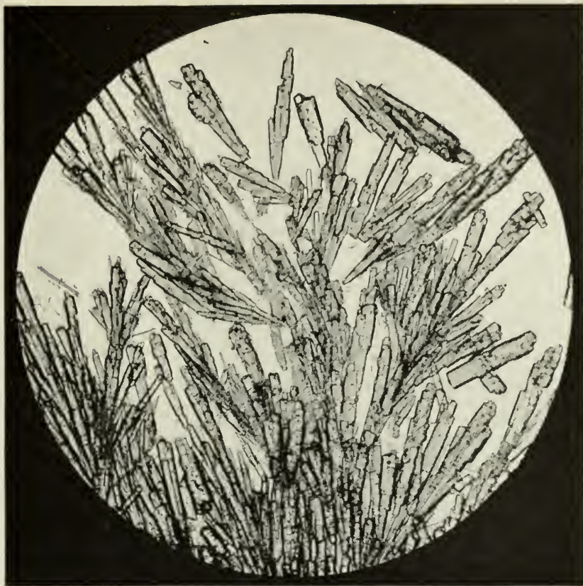
FIG. 1.—CRYSTALS OF LARD TO WHICH 10 PER CENT OF COTTON-SEED OIL WAS ADDED. \times 100 .
