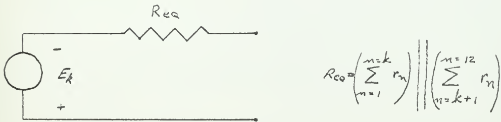
FIG. II. 8 EQUIVALENT CIRCUIT OF BIAS CHAIN AT k th BIAS POINT ABOVE GROUND.
