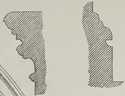
Section of Cap and Base 2 nd Scale
