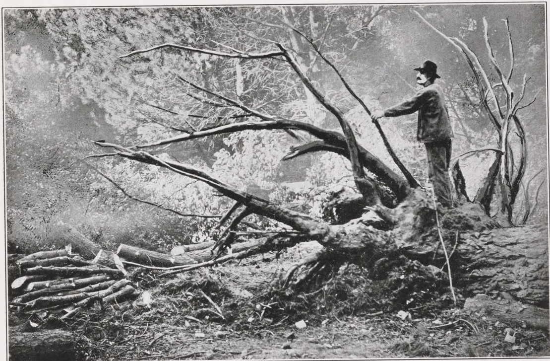
A fair example of the tremendous power of the 90-ton horse-power Bull Dog. One root of this 34-inch fir stump was 36 feet long, and another root was 16 inches in diameter. But they came out in 17 minutes, with the stump , although they were firmly embedded in dry soil. Still "Daddy" Cole, seen in the picture, will tell you that the Bull Dog never "weakened"
