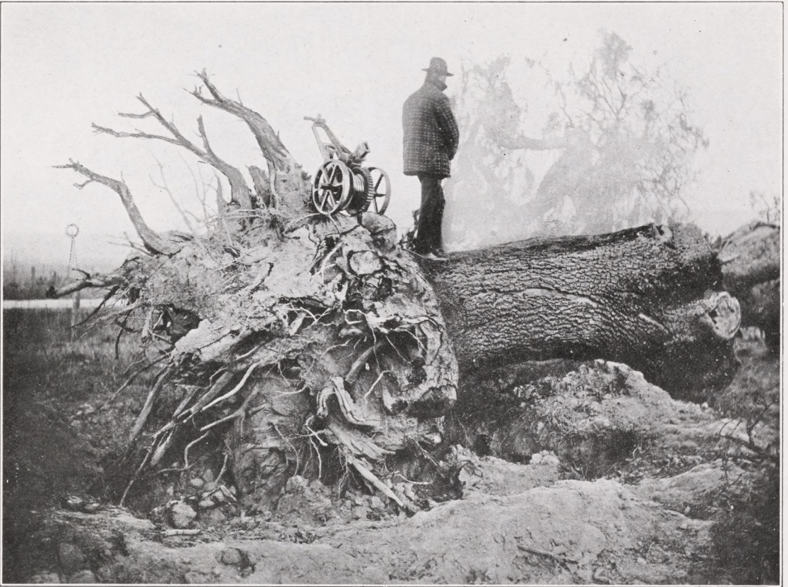
It is hard to believe, but the Bull Dog Hand-Power Machine, weighing only 175 pounds, pulled this sturdy oak, four feet in diameter, in twelve minutes. John Southers, who is shown in this picture, says that he can pull even larger ones
