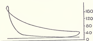
Fig. 27. Indicator Card with Too Early Ignition.
