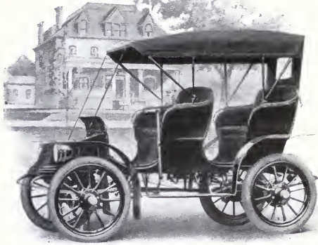
Fig. 159. Baker Electric Surrey, with Cape Top. Can be quickly converted into an inclosed vehicle in stormy weather. Baker Motor Vehicle Company, Cleveland, Ohio.
