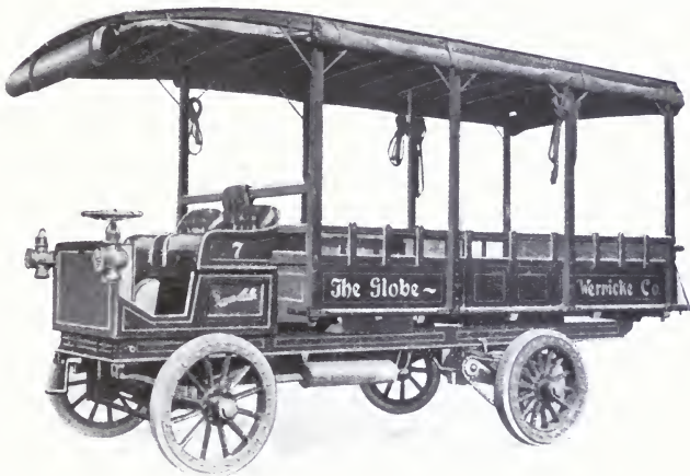
Fig. 180. Frayer-Miller Motor-Truck. For delivery of furniture or other bulky and heavy goods. Oscar Lear Automobile Company, Springfield, Ohio.
