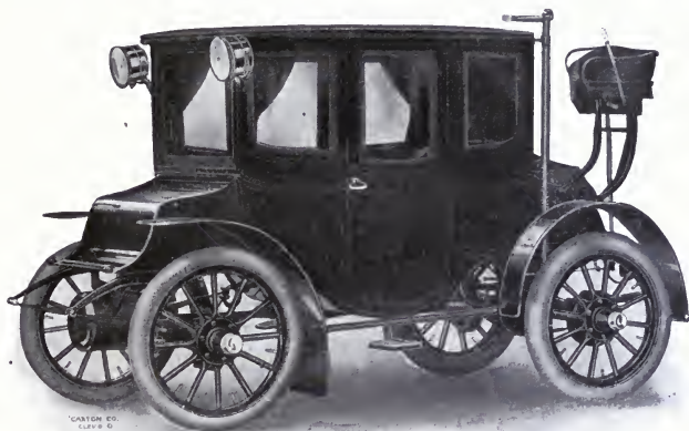
Fig. 158. Rear-Driven Brougham. A type now superseded by the front-driven Brougham. Baker Motor Vehicle Company, Cleveland, Ohio.
