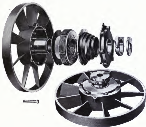
Fig. 99. Multiple-Disc Clutch of the Franklin Car. H. H. Franklin Manufacturing Company, Syracuse, N. Y.
