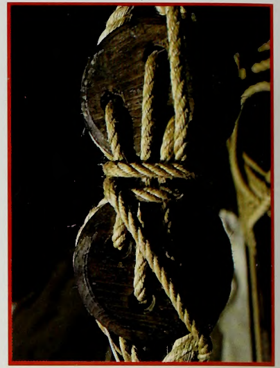
Large wooden deadeyes connect the shrouds, the heavy ropes that hold the masts up, to the deck.
