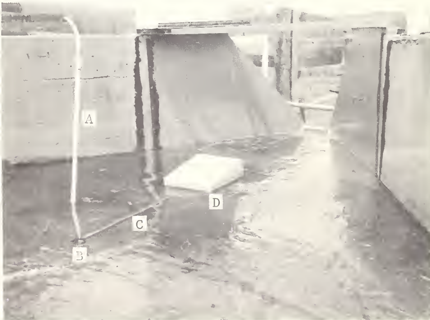
Figure 7.--Sample intake system in water. A , Suction tube leading to pump; B , anchor; C , intake sampling tube; and D , float.
