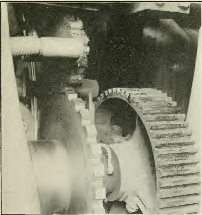
Milne Peat press, showing die- or sprocket-wheel in which briquettes are compressed.
