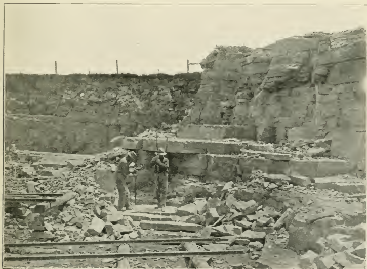
Horseshoe Quarry, St. Mary's. Product used for building—rubble, sills and courses; and waste rock for road metal. Perth County.
