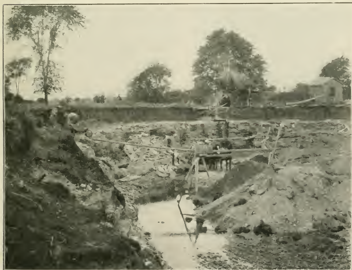
Limestone quarry at Beachville. Product used in making lime for building and refining beet sugar. Oxford County.
