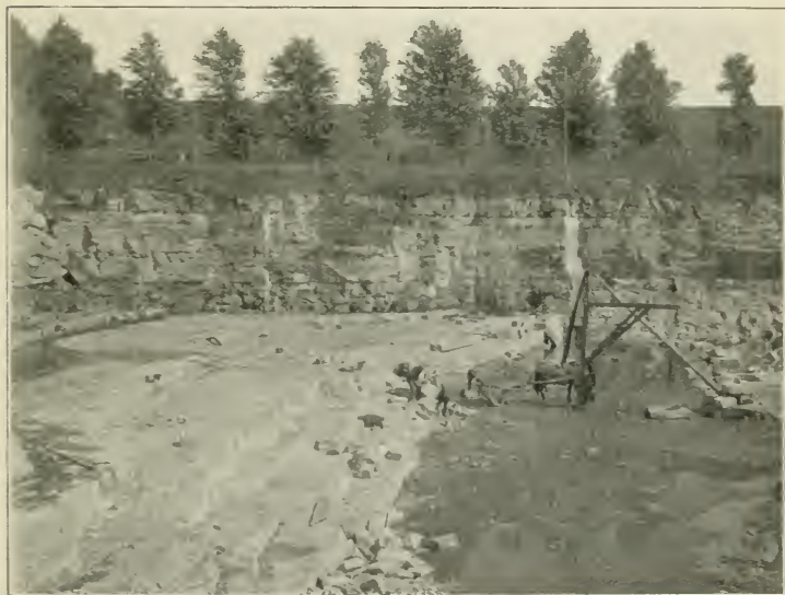
St. Marys quarries. Product used for building, and waste rock for road metal. Opening is 200 by 400 feet, and 20 feet deep. Perth County.
