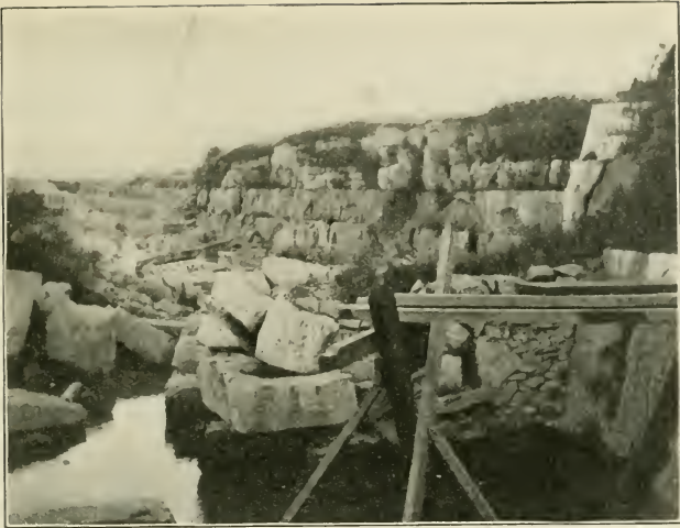
Gray dolomite bluff, Anderdon quarries, showing debris from quarrying block stone. Essex County.
