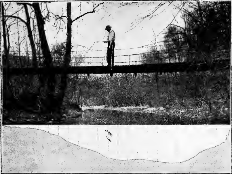
FIG. A.—Method of making a measurement of the amount of water in a stream, using current meter from bridge.
