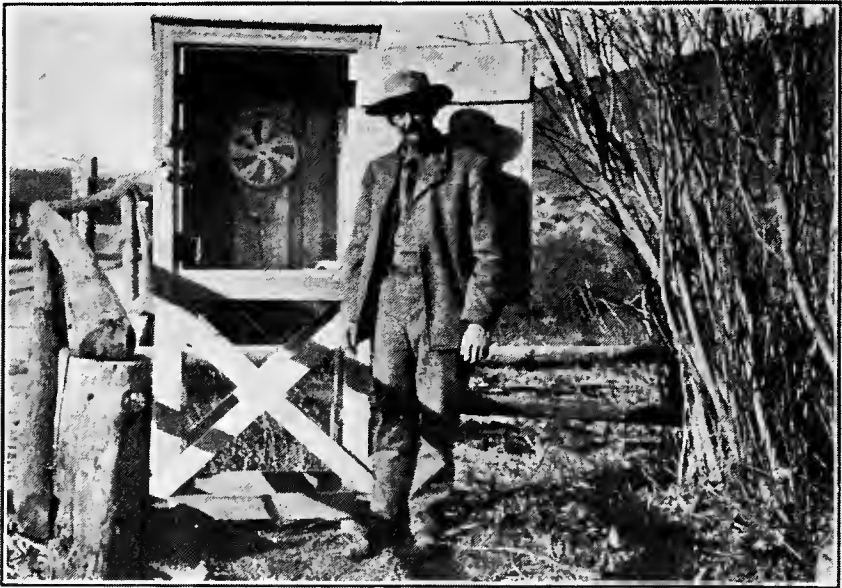
FIG. D.—Automatic gage for recording height of water in river or main canal. Laramie River, Colo.
