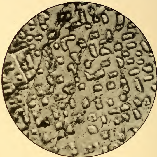
Fig. 7.— Intergrowth of diopside (square and rectangular outlines) and scapolite, Lower Albion, Hakgala. × 120.
