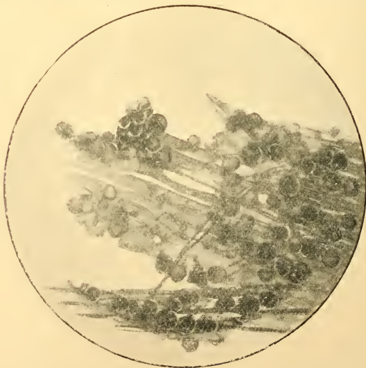
Fig. 4.— Nodules of calcium-carbonate, growing upon wood treated alternately with sodium-carbonate and calcium-chloride solutions.
