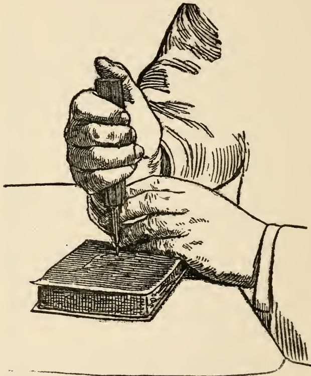
FIG. 16.—USING A HAND PUNCH
