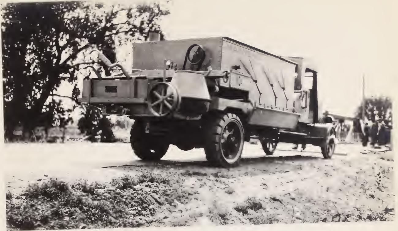
A MAINTENANCE TRUCK USED BY THE COLORADO STATE HIGHWAY DEPARTMENT CARRIES MATERIAL BINS AND A CONCRETE MIXER
