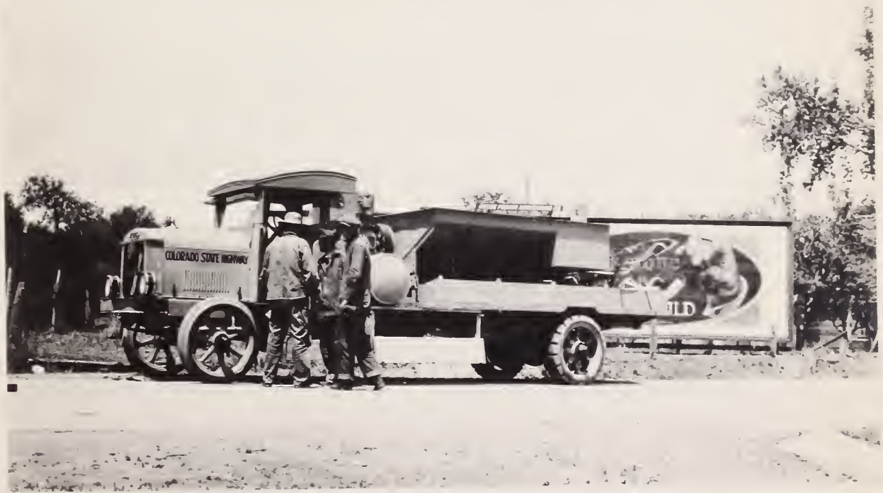
THIS TRUCK IS EQUIPPED WITH AN AIR COMPRESSOR. THE BODY WILL HOLD A PLOW AND SMALL SCRAPER. THERE IS A TOOL BOX UNDER THE MATERIAL BINS
