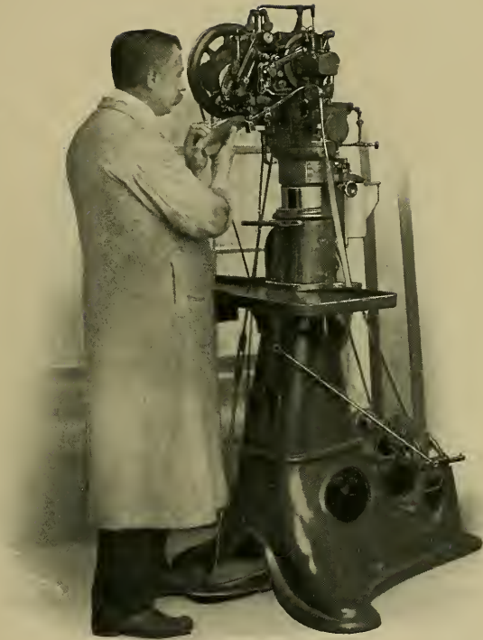
Operating the Goodyear Welt Sewing Machine
