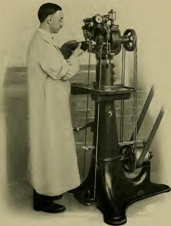
Operating the Goodyear Rough Rounding Machine
